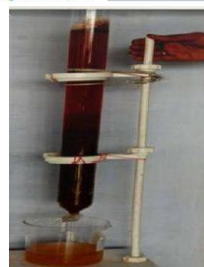
Adsorption of anthocyanins by using an adsorbent (XAD-16)
